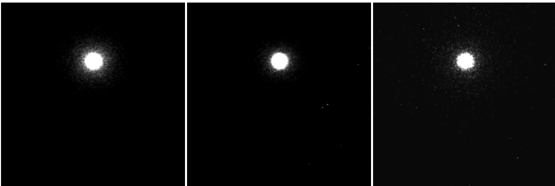
Figure 18: Reconstructed images of the mouse-like NEMA phantom using the list-mode MLEM code. Images represent the normal threshold method (left), the true Geant4 data (center), and the Compton weighting scheme (right). Reduction in scatter directly surrounding the source is apparent in the weighting method image.
