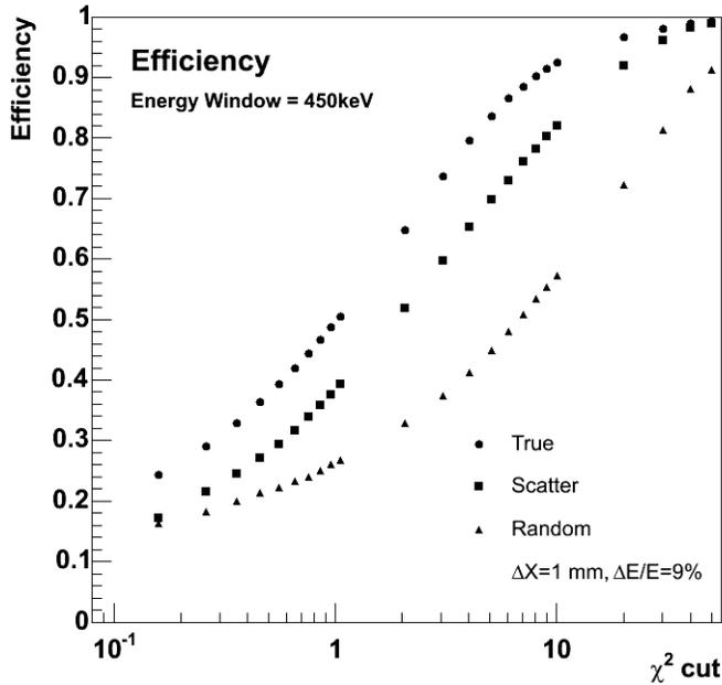
Fig. 3. Normalized efficiency vs.  $\chi^2$  of the Compton reconstruction algorithm for true, scatter, and random events at 70 MBq. The difference in efficiency allows background suppression via an upper  $\chi^2$  threshold cut.
