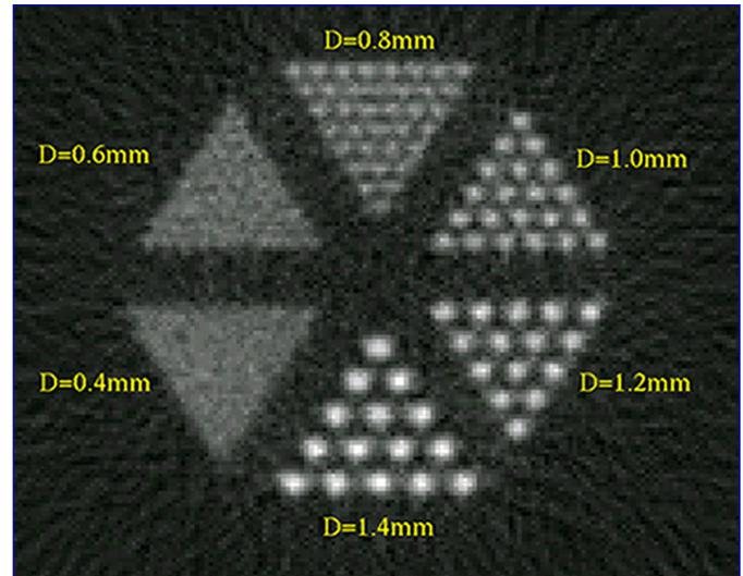
Figure 4: Image reconstructed for a simulated micro-Derenzo image contrast phantom with source rods of various diameters immersed in a 6 cm diameter water phantom. Rod-to-rod separation was equal to twice the associated rod diameter. The image was reconstructed using a Filter-Back Projection algorithm [7] with a modified Ramp filter having a cut-off at the Nyquist frequency. The data count rate was equivalent to a 20 min scan at 1 MBq total activity.
