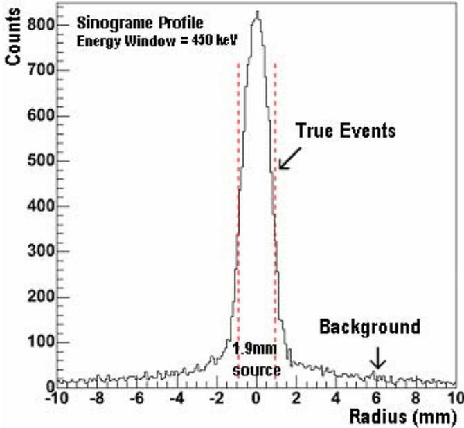
Fig. 2. Sinogram profile of a 1.9 mm diameter 1 mCi water line source inserted into the rat size phantom at a 15 mm offset from the center. Sinogram projections were centered on the source peak and combined. All true events were assumed to be within a 9 mm narrow band centered on the source peak. Background events within the narrow band were assumed to be constant and interpolated as the average of the counts at the edge of the narrow band.
