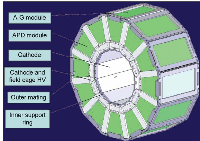
Fig. 1. Schematic drawing of the simulated LXe PET system.
