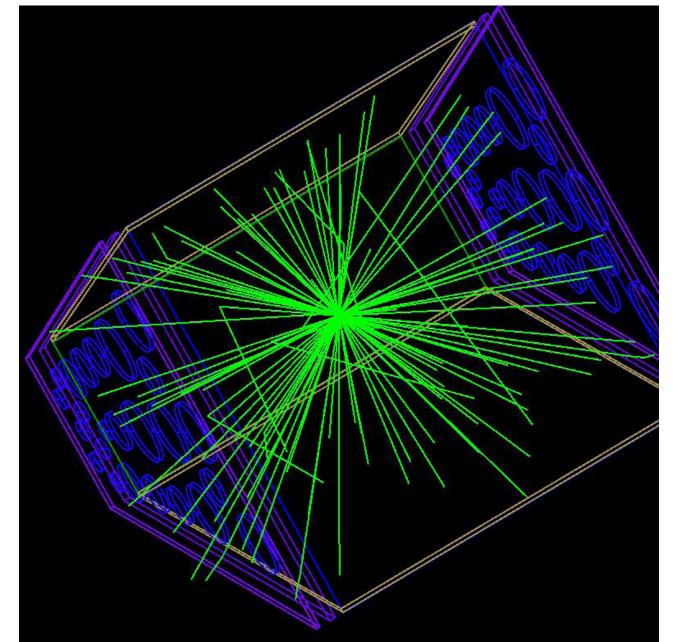
Figure 2: Simulation of a scintillation event in the center of the chamber. The number of optical photons reaching the surface of the LAAPDs are
