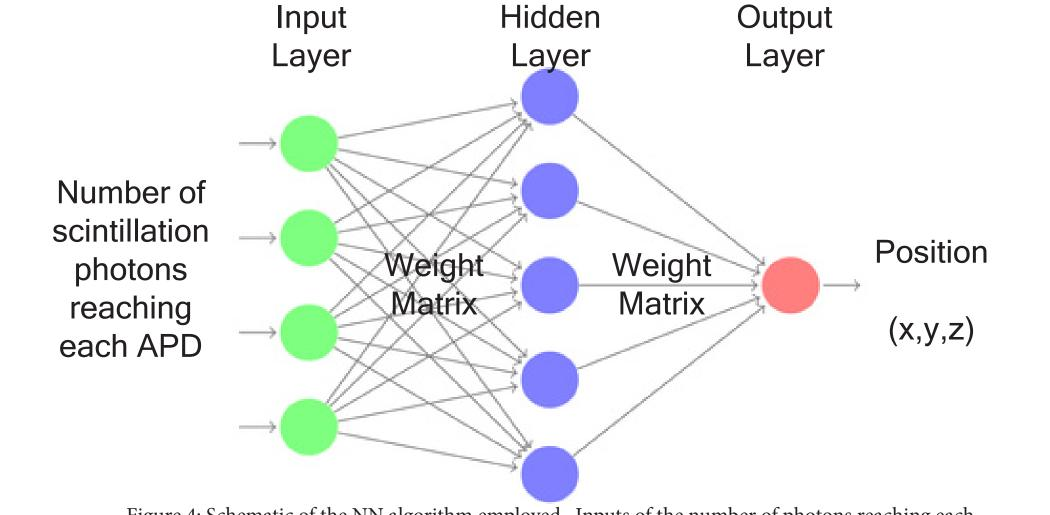
Figure 4: Schematic of the NN algorithm employed. Inputs of the number of photons reaching each APD are evaluated with 160 hidden layers to find the position of scintillation within the sector.
