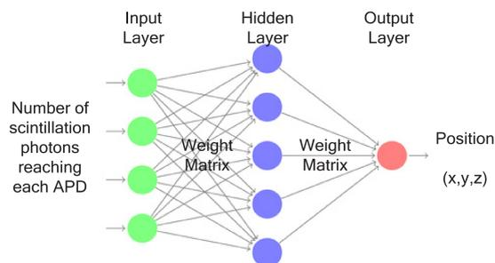
Figure 4: Schematic of the NN algorithm employed. Inputs of the number of photons reaching each APD are evaluated with 160 hidden layers to find the position of scintillation within the sector.
