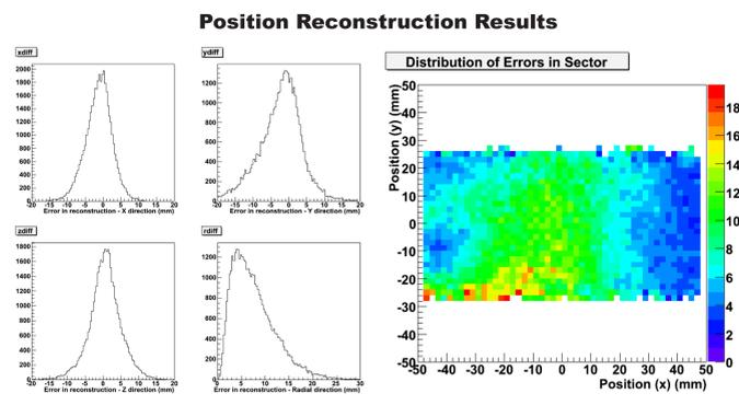
Figure 5: Reconstruction results for the case of no reflectivity within the sectors. Reconstruction error generally increases towards the center of the sector, away from the position of the APDs.
