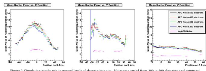
Figure 7: Simulation results with increased levels of electronics noise. Noise was varied from 200 to 500 electrons and compared to the case with zero electronics noise applied.
