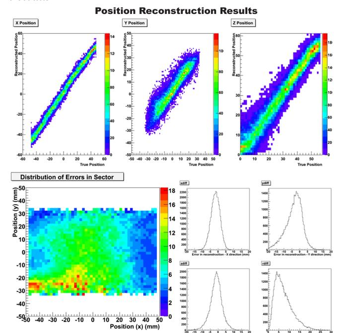
Figure 6: Reconstruction results for the case with reflective surfaces added to the sector configuration. The position reconstruction improved slightly over the zero-reflectivity case.
