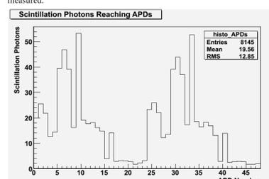
Figure 3: Histogram of the number of photons reaching each LAAPD from a scintillation event of 10220 photons generated at the center of a LXePET sector.
