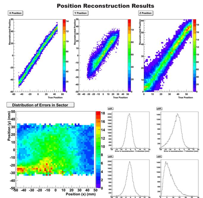
Figure 6: Reconstruction results from the case with reflective surfaces added to the sector configuration. The position reconstruction improved slightly over the zero-reflectivity case.
