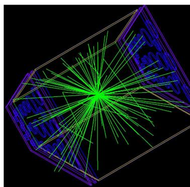
Figure 2: Simulation of a scintillation event in the center of the chamber. The number of optical photons reaching the surface of the LAAPDs are measured.
