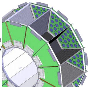
Figure 1: Schematic of the LXePET prototype. The prototype consists of 12 concentric TPC sectors filled with liquid xenon. LAAPD detectors are shown on the inner walls of the sector.
