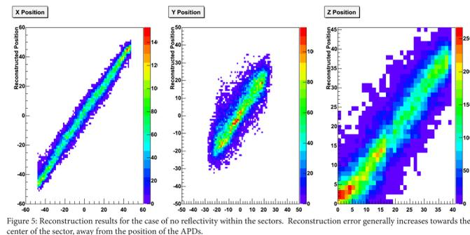
When electronics noise of 500 electrons is applied to the APD signal, the resolution is degraded to approximately 9.0 mm FWHM in 3 dimensions.
